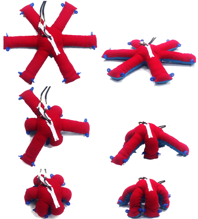
Fig. 8. Fabricated hexapod example with no legs contracted (top), one set of legs contracted (middle), and both sets of legs contracted (bottom), shown from a top view (left) and a side view (right).
