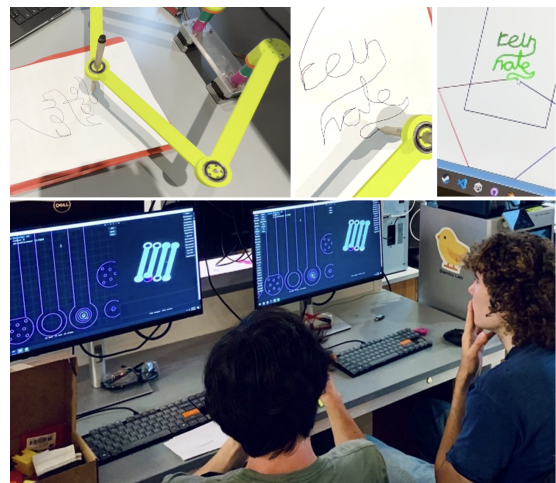
Figure 1: Five-Bar Linkage Arm by Anonymous Students; course final project. A team of two students independently designed this yellow five-bar linkage robotic arm in SplitCAD. The arm is shown writing their names (“rein” and “nate”) in cursive. The stepper motor assembly was designed by the primary author, also in SplitCAD.
