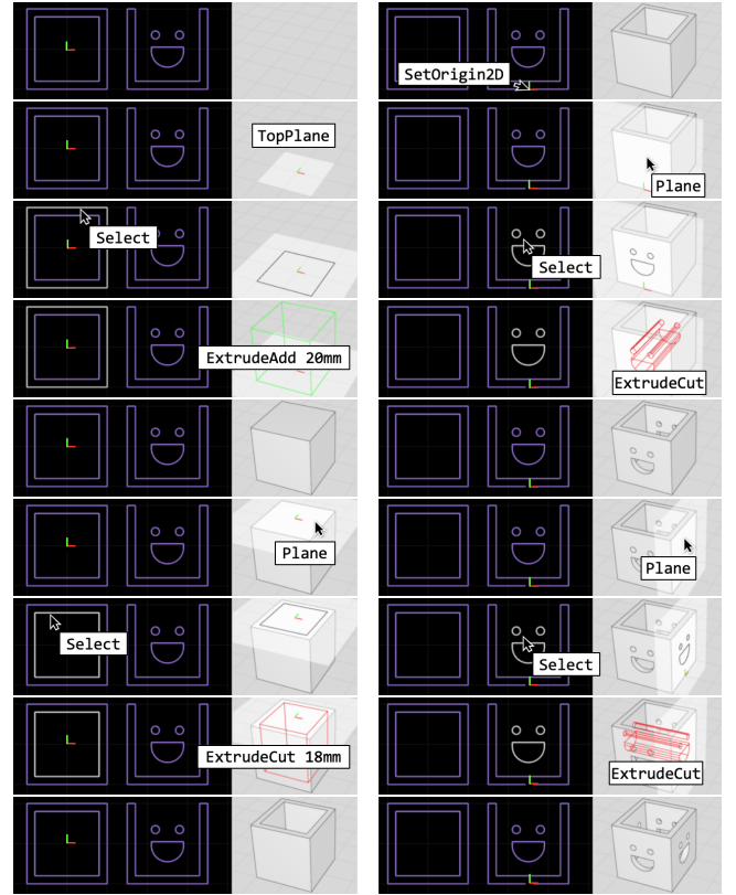
Figure 5: Annotated sequence of screenshots of a user modeling Happy Box in SplitCAD, starting from a single sketch of the box’s top and side views (shown in purple). Reading column by column, the user first chooses the world top plane to be the current feature plane, and selects the outer contour of the box’s top view (shown in white). The user then extrudes the box up (preview shown in green wireframe). The user then selects the top of the box as the current feature plane, selects the inner contour of the box’s top view, and cuts down into the box (preview shown in red wireframe). The user then snaps the 2D origin to the middle of the side view’s bottom line, selects the smiley face, and cuts through the box’s sides. Finally, the smiley face cut is repeated using another side of the box as the feature plane.
